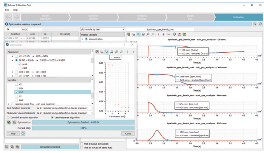
Figure 1: Simcenter Amesim Exhaust calibration tool is an interactive interface with a step by step workflow
