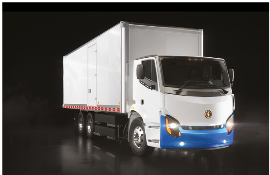
Figure 3: All-electric Urban Class 8 truck
