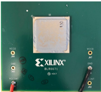
Figure 1: Xilinx Package mounted on JEDEC 2S2P PCB
