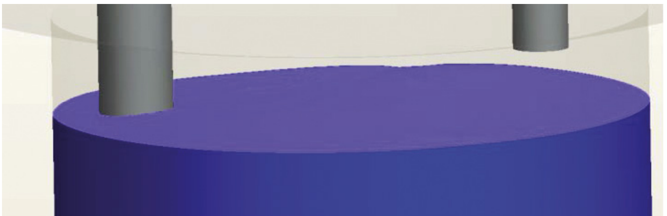
Figure 7. The air-water interface in the sump, showing a low level of deformation, indicating no vortex formation or air entrainment
